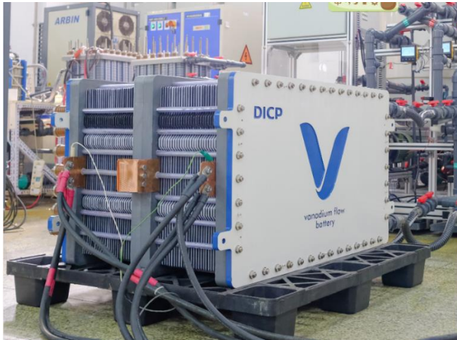
Previous generation 30kW stack
