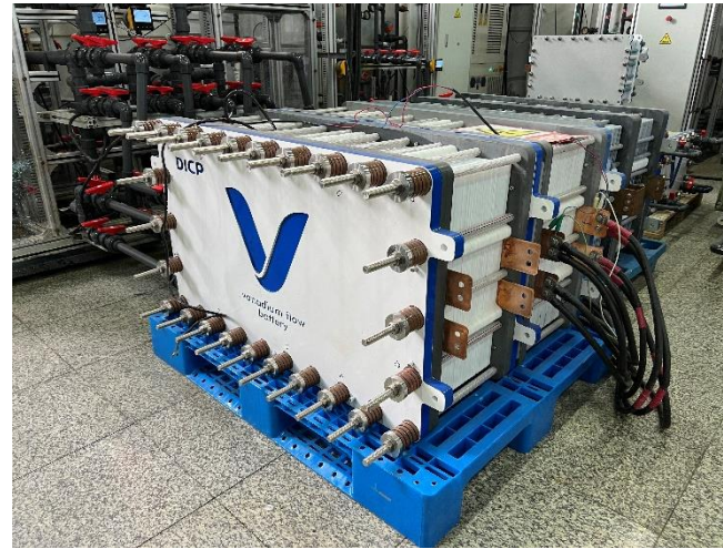
New design 70kW stack
