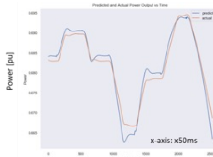
RTDS PSH model output power prediction using reservoir computing (left); and ROR hydro power prediction using machine learning in Tensorflow2 (right)
