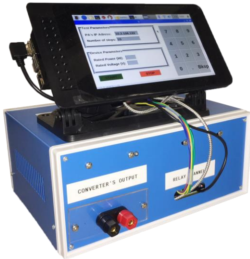
Controllable Load Bank, 20V, 400W.
