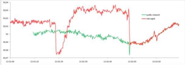
Measured phase difference between the microgrid and the public network.
