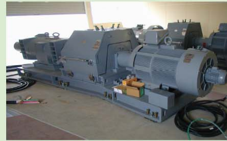
150kW rotating type generator (simulates WP, Co-generation)
