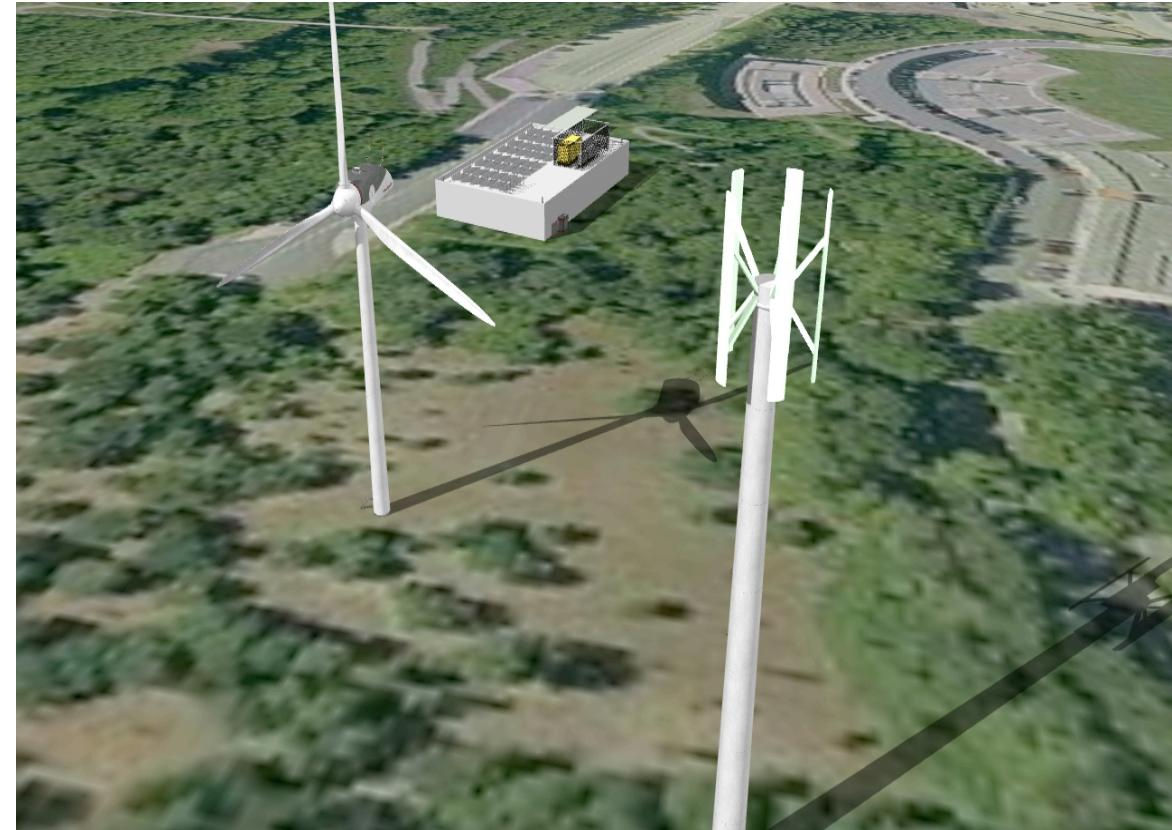
Horizontal and vertical axis wind turbines
