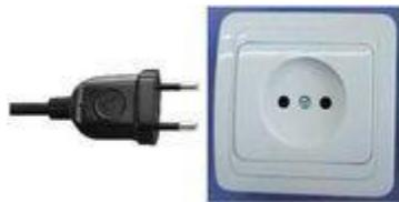
Type C plug (Europlug) The plug is non-earthed and has two round 4 mm (0.16 in) pins, which usually converge slightly towards their free ends. It can be inserted into any socket that accepts 4 mm round contacts spaced 19 mm (0.75 in) apart.
