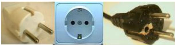
The type F plug, commonly called a "Schuko plug", has two earthing clips on the sides of the plug instead of a female earth contact. The Schuko connection system is symmetrical and unpolarised by design, allowing live and neutral to be reversed. The socket also accepts type E plugs and Europlugs. It supplies up to 16 A.
