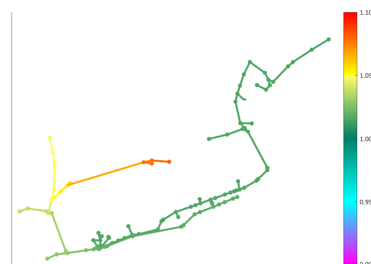
Figure 3: Heat map of voltage profile showing voltage rise on Feeder 1 where the PV is connected.
