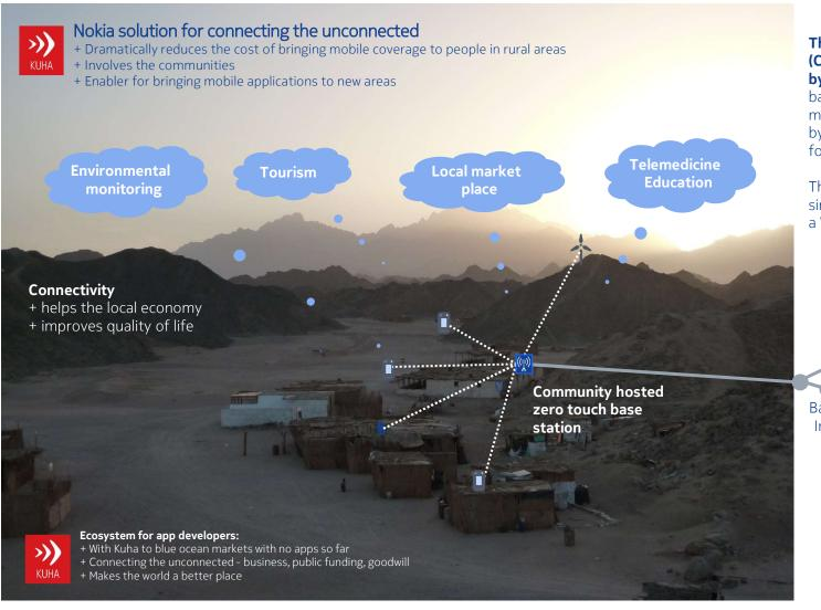
The target is to reduce the cost (CAPEX) of building rural coverage by 90% when compared to macro based solutions and to reduce maintenance cost (OPEX) by > 75% by enabling communities to care for their base stations.
