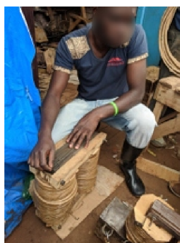
Fig. 2: Handmade arc welder (Kigali, Rwanda, 2018).
