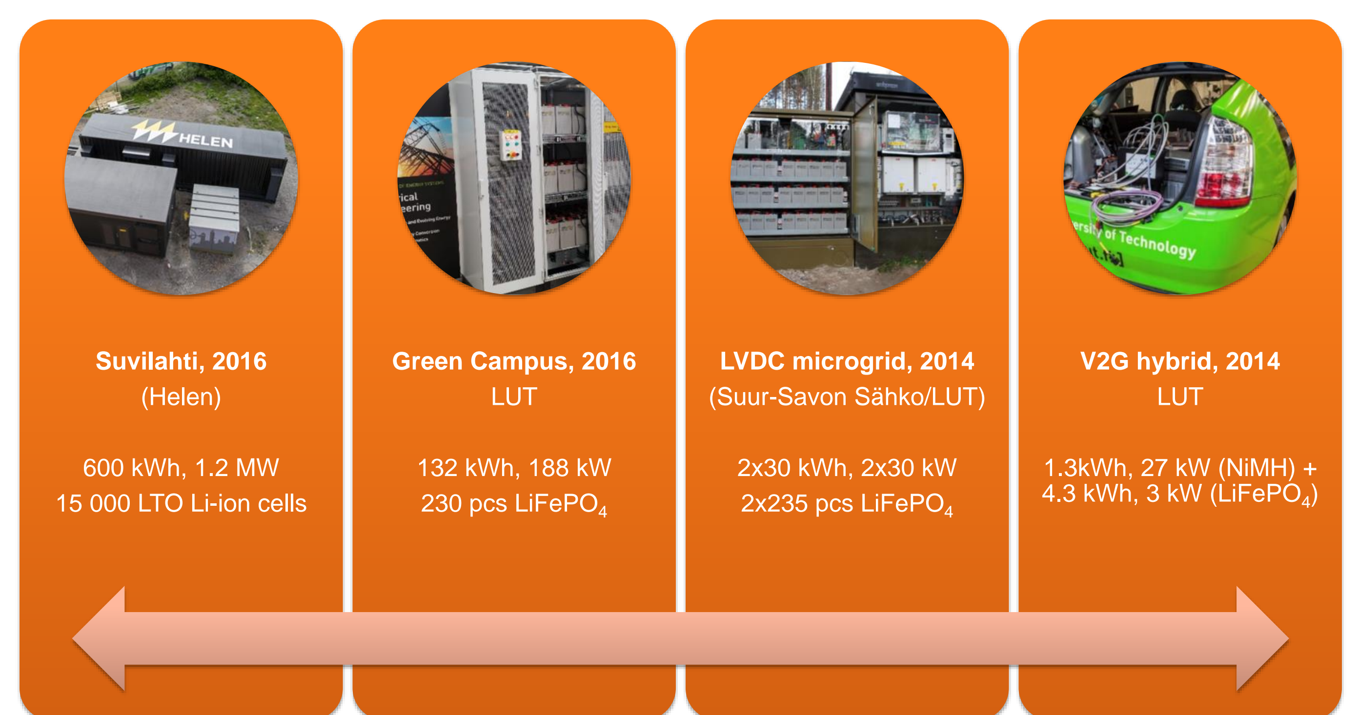
Figure 3. Characteristics of BESS in each test site.
