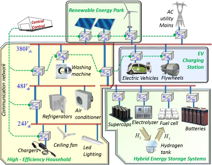
The DC bus is the "dorsal spine" of any DC distribution system, therefore, its voltage stability and control should be considered as a critical issue.
