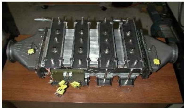
330W waste heat generator of engine gas
