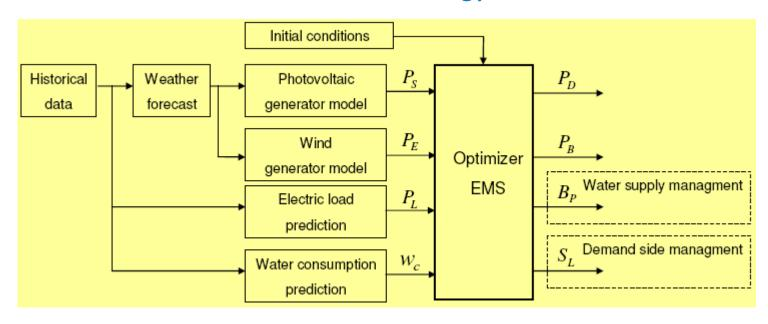
References for the diesel power  $(P_D)$ , the battery power  $(P_B)$ , the signals for the water supply system  $(B_P)$ , and the signals for consumers  $(S_1)$ .
