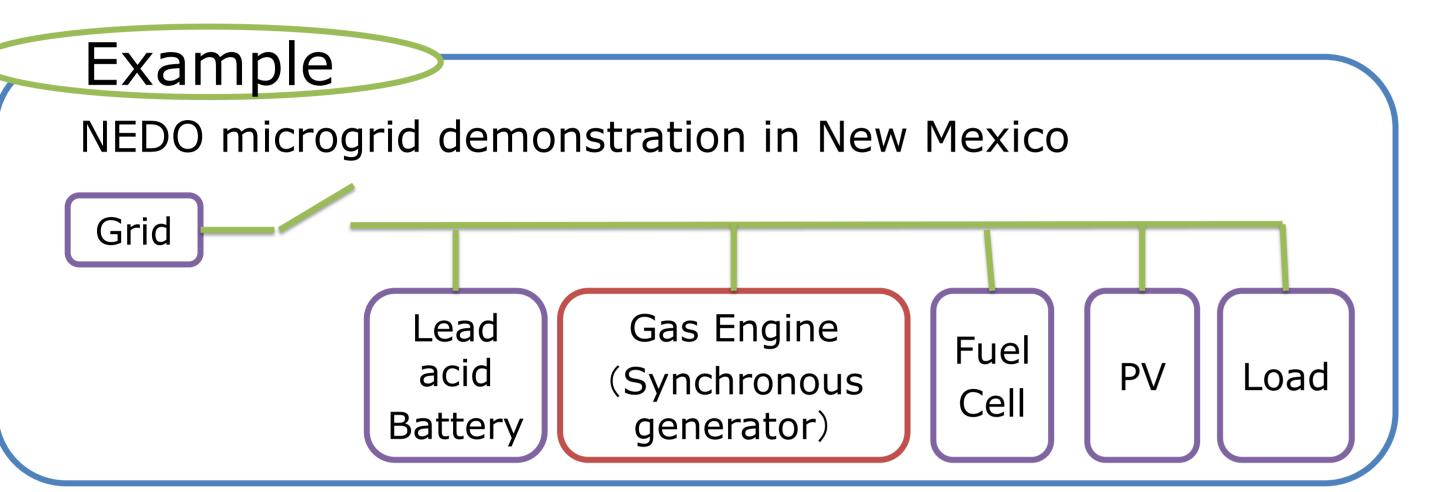
These Microgrids require the synchronous generators to operate since the synchronous generator maintained the microgrid voltage and frequency.
