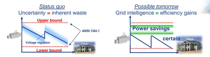
Optimize Voltage and VAR profiles to minimize distribution losses and manage load
